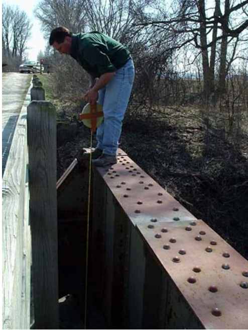
Photo 5A. Mouth of the Bonne Femme & Missouri Rivers at walking bridge where the survey was taken. Looking at cross-section surveying technique of locations only accessible via a bridge locations. See Excel Spreadsheet under Photo 5, “Location.”
